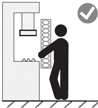
Fig 3.1.1.2 The hazardous zone of a machine can be reached only by passing through the sensor's detection zone.
