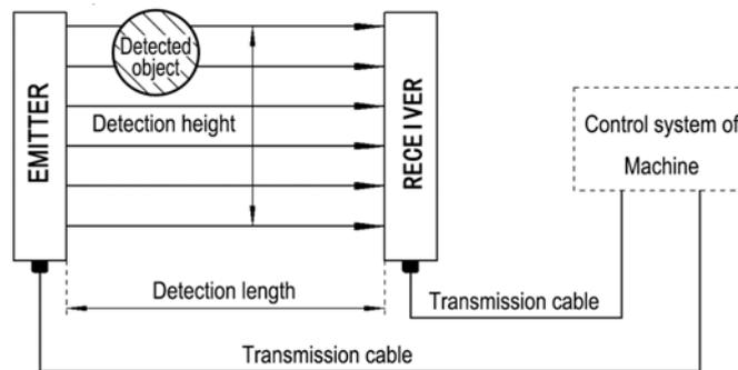
Fig 1.4 Operation schematic diagram
