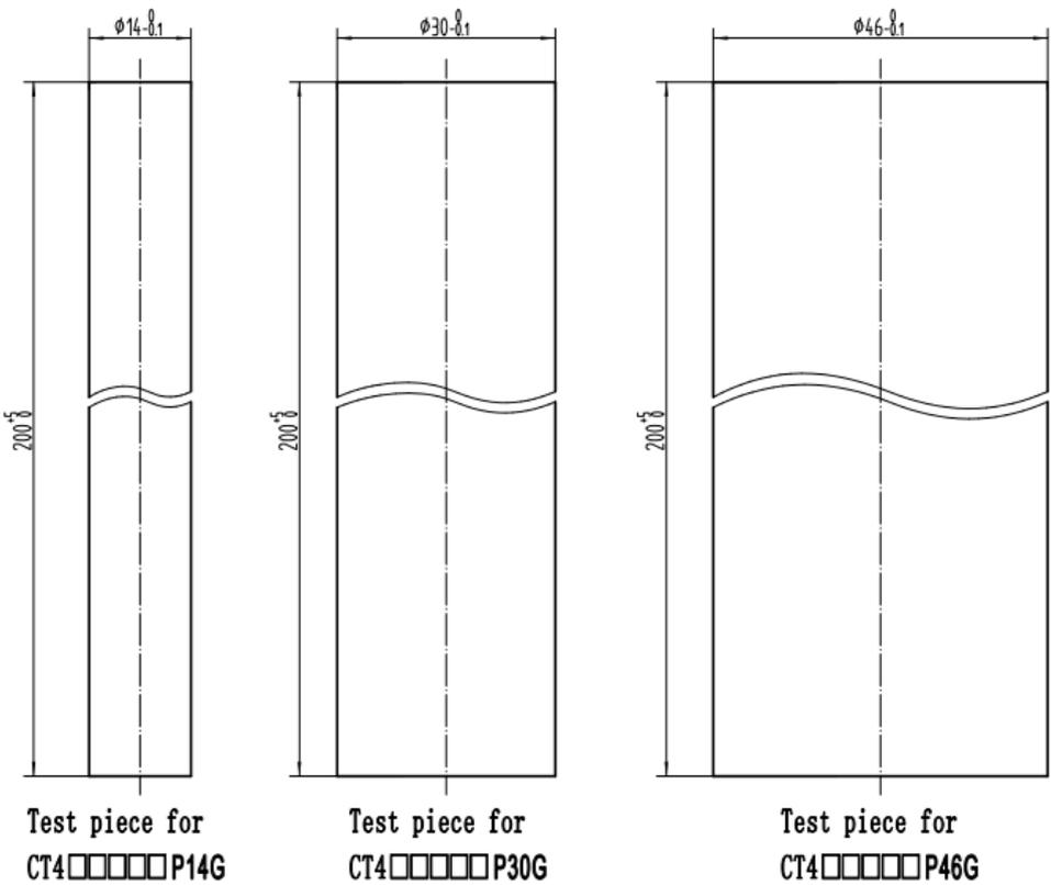
Fig. 1.9.1 Specimen Specification Diagram (Unit: mm)
