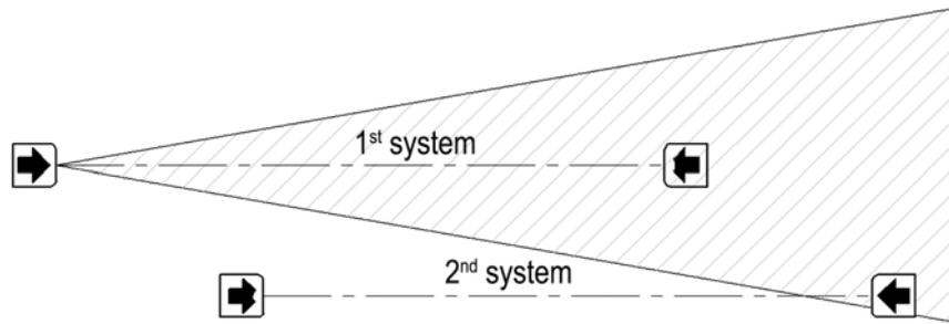
Figure A.2 Reversing the transmission direction of systems in close proximity.
