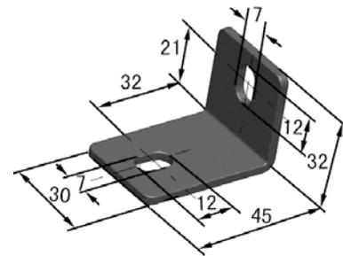
Fig 1.8.3 L-shaped Bent Plate Bracket
