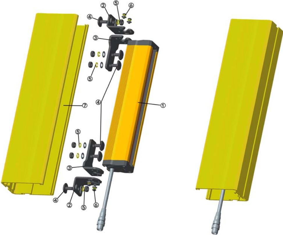
Fig 3.2.1.5 Scatter shield mounting diagram
