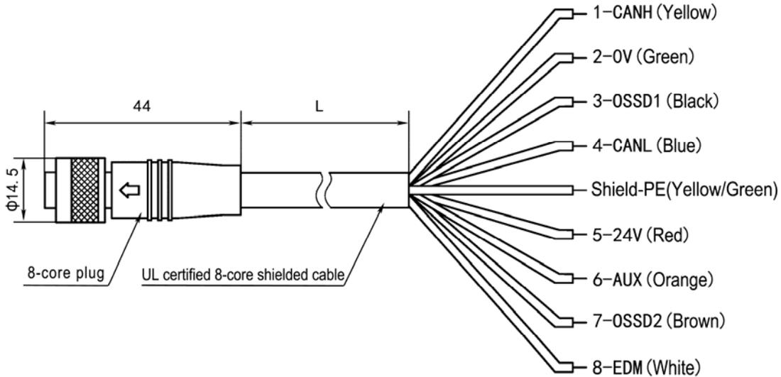
Fig 1.3 Schematic Diagram of Connection Points of CT4 Secure Grating Transmission Cable
