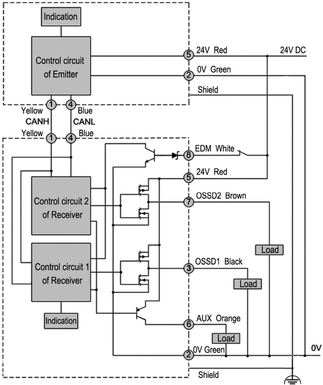
Fig 2.1 Input and Output Interface Circuit Diagram
