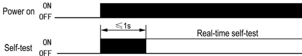
If an error is found in the self-test, the CT4 enters lockout state, keeps the OSSDs in OFF-state, and indicates the error at the same time. After the error is removed, only through re-power can release the lockout state .
