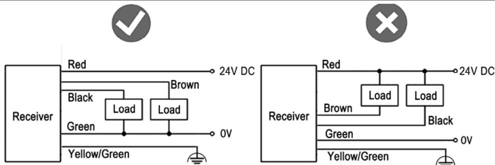
Fig 3.3.1 Schematic Diagram of Correct and Error Load Wiring
