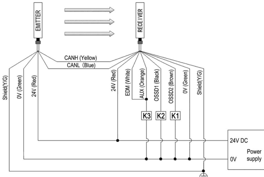
K1 · K2 : Relay or other device that controls hazardous parts of the machine
