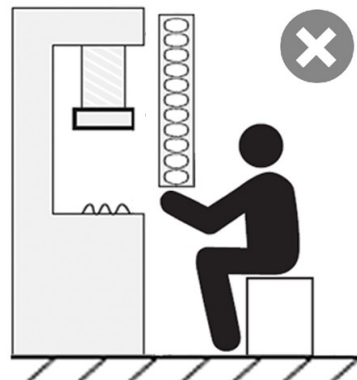
Fig 3.1.1.5 The operator can reach the hazardous zone of a machine through the lower zone to the sensor's detection zone(the ESPE is too high).
