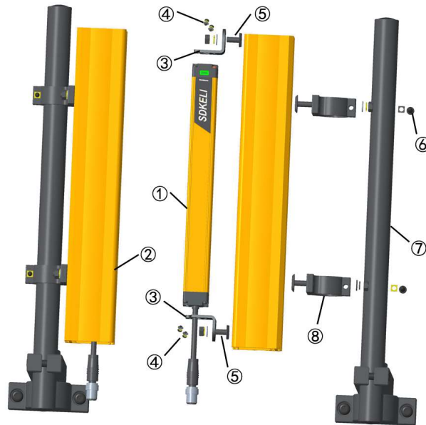
Fig 3.2.1.8 Scatter shield pipe mounting diagram(GF)
